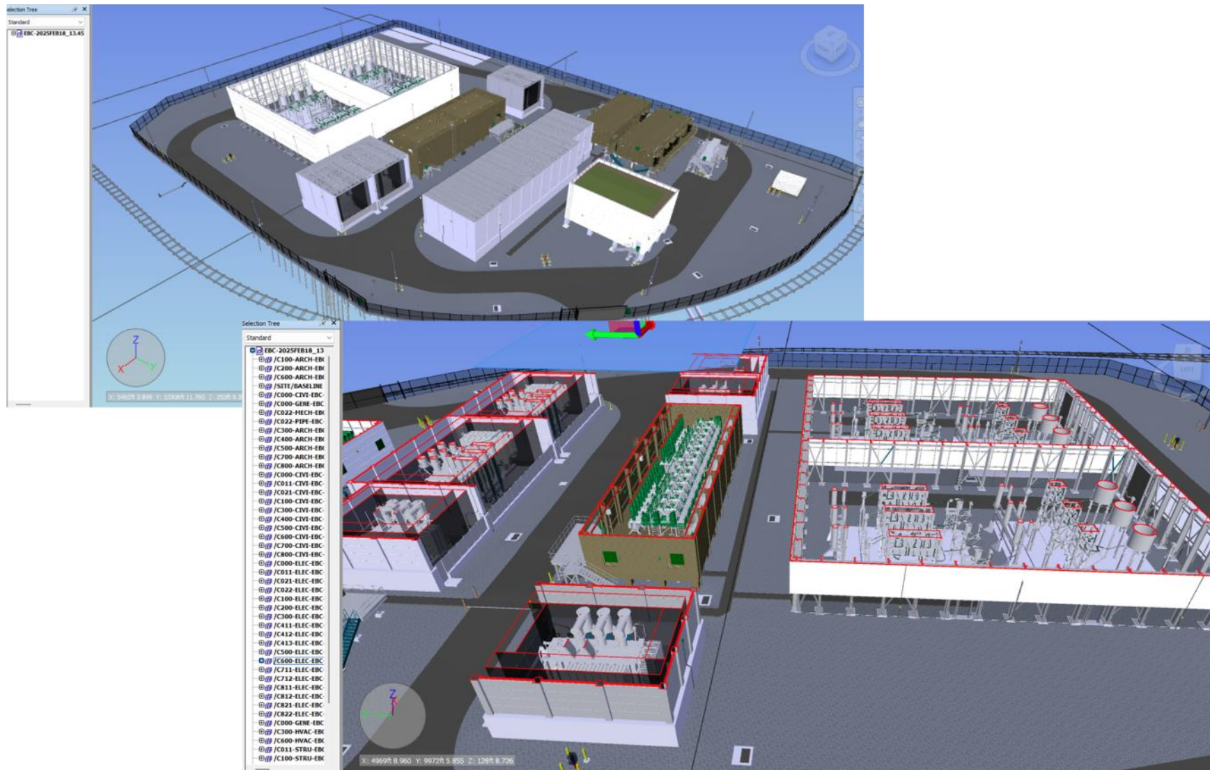
Electric wind power generation facilities, located in Quebec, Canada, in the rapid modeling of information provided in 2D files by mechanical equipment suppliers, and providing files compatible with the project's 3D model system.
